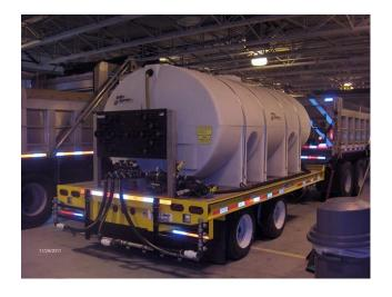
PennDOT will use an 8,000 gallon salt brine tanker (pictured above) to spray brine on three travel lanes. The truck operates on I-76, I-476 and Route 422 in Montgomery County. When operational, it can spray salt brine on all three expressways without being refilled. When the large tanker is not spraying brine, it is used to fill salt brine tanks at other state stockyards in Montgomery County. PennDOT District 6 has another tanker truck that holds 2,600 gallons of brine.
