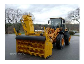
PennDOT will use a snow blower that is capable of moving up to 1,200 tons of snow per hour. The snow blower is mounted on a front loader and used in areas where drifting snow is prevalent.
