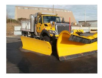
PennDOT will use double wing plows to push snow and ice off state highways. This specialized truck is outfitted with wings on both sides of the plow that extends and can clear up to 21 feet of snow at a time.
