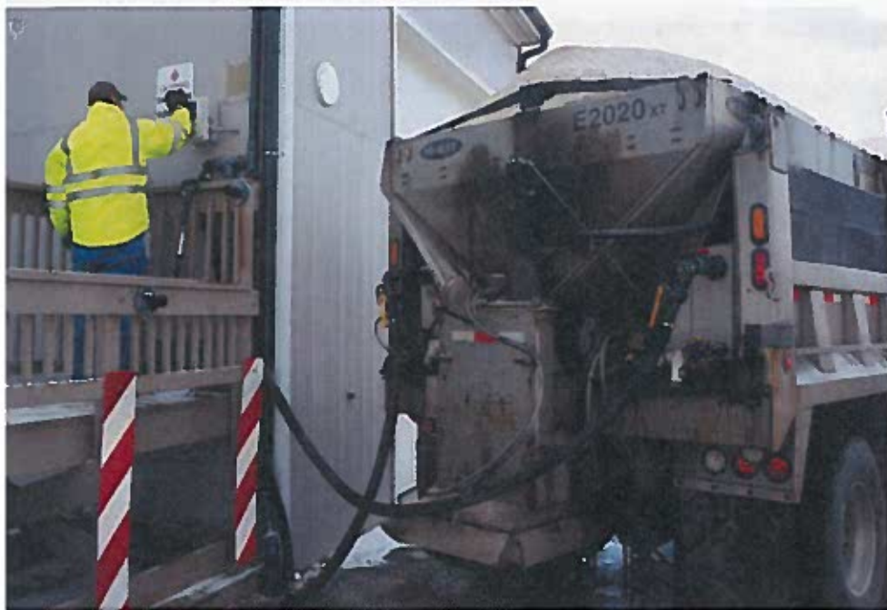
A member of the public works crew in Cranberry Township, Butler County, fills the brine tank on a salt truck. The brine will be used to prewet the salt as it is applied to the roads. (Photo courtesy of the township.)
